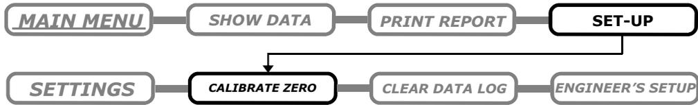
Tare Zero Weight is used to set the "No load" point on each of the perches. The function is mainly used during calibration which is described in greater detail in section TARE ZERO WEIGHT AND CALIBRATION but is also used to simply make the display read zero should the need arise.
